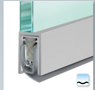
Option: Planet KG-U, bevel lip for uneven floors
